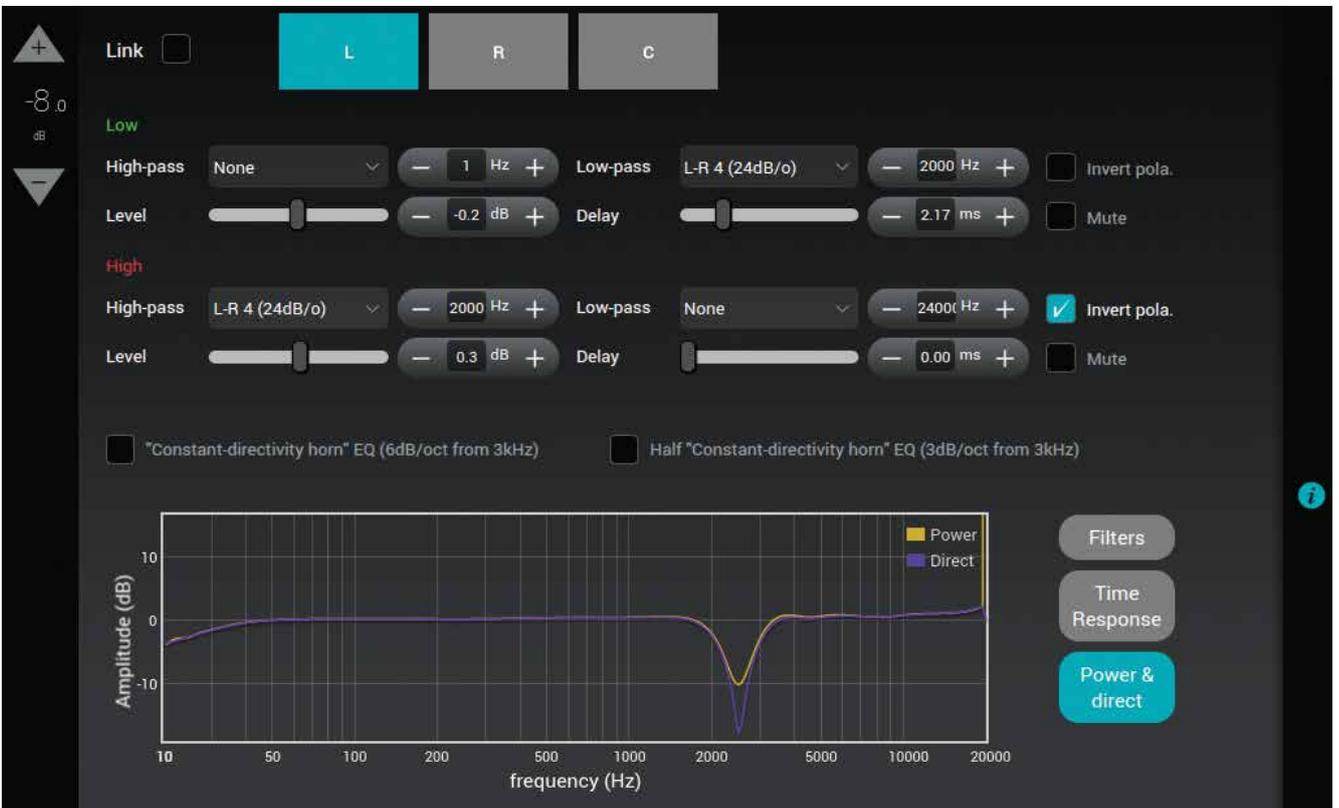
Figure 79: frequency response (power and direct)
