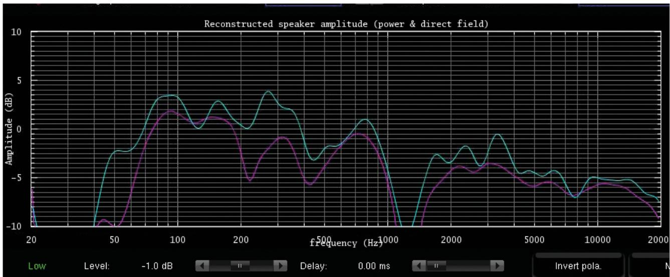
Figure 126: Recombined amplitude response of the speaker
