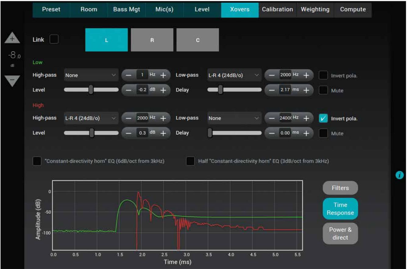
Figure 78: Measured time response of both drivers
