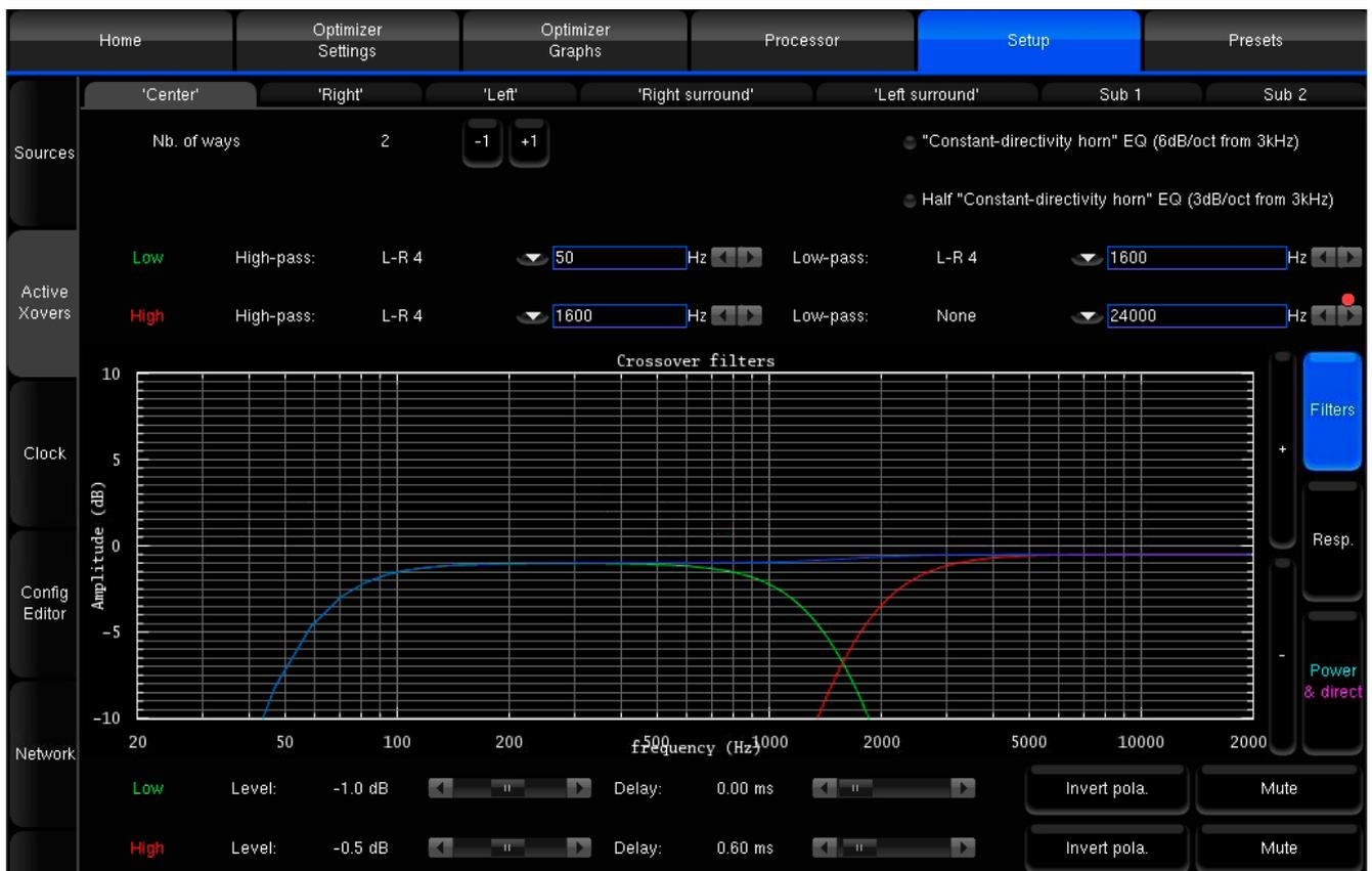
Figure 127: Performing the calibration of the active crossovers
