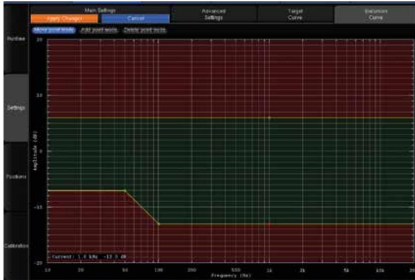
Figure 113: example of a limiter curve for maximum boost/attenuation
